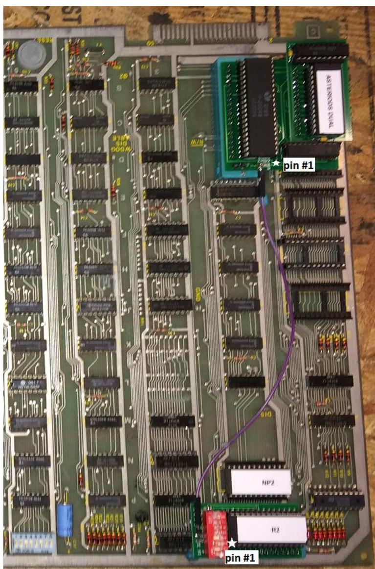
Figure 3 – Image of installed ASTDELUXE-DUAL-CB
