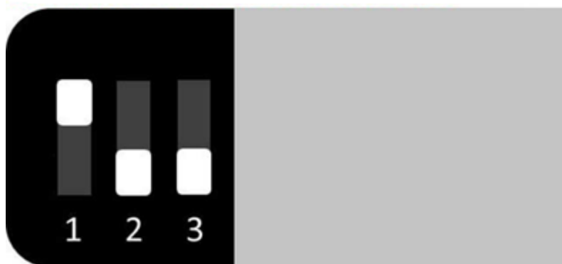
Figure 6 - Settings for installing the SRBP in a 2516 or 2716 ROM socket
